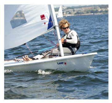
Photo caption: Laser's dinghies have an FRP composite hull and deck, designed and manufactured by LaserPerformance in the UK, North America and China using high performance, marine approved resins, gelcoats, core bonding and structural adhesive materials from Scott Bader.
